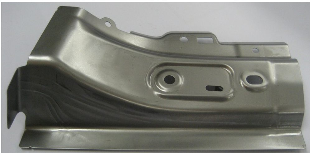
Fig. 1 Internal reinforcement of car bodyshell B-pillar.
