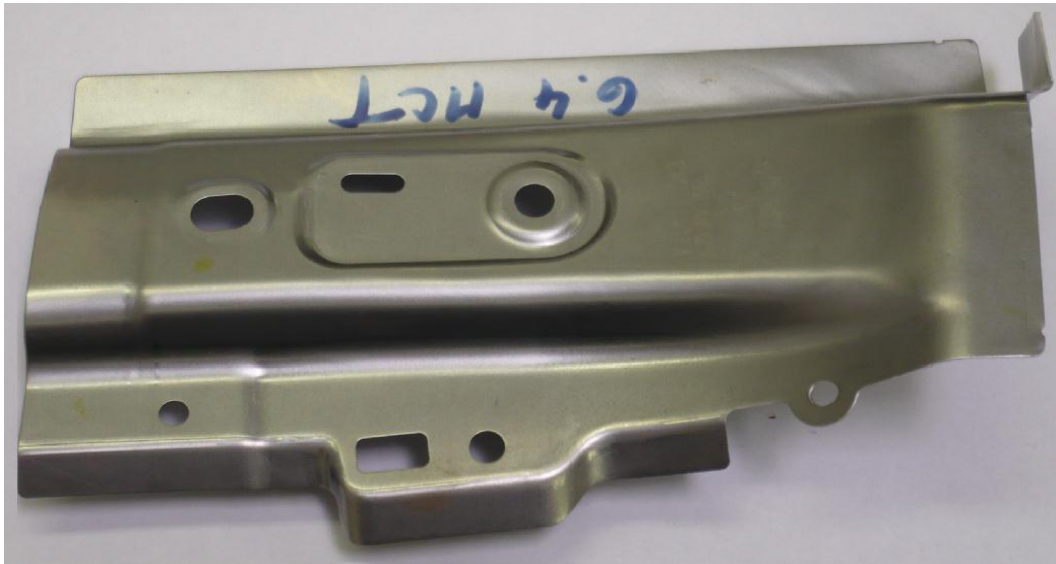
Fig. 1 Internal reinforcement of car bodyshell B-pillar.
