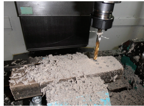
FIGURE 2: Holes with required diameter drilled into the material.
