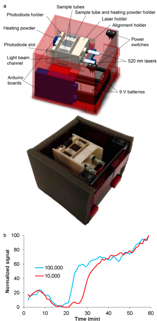
Figure 6. Homemade prototype device for real-time LAMP assay. (a) Schematic (top) and photograph (bottom) of the homemade prototype device. (b) Plots of photodiode signal versus LAMP reaction time using the homemade prototype device for samples containing 10 000 and 100 000 copies of lambda DNA target.
