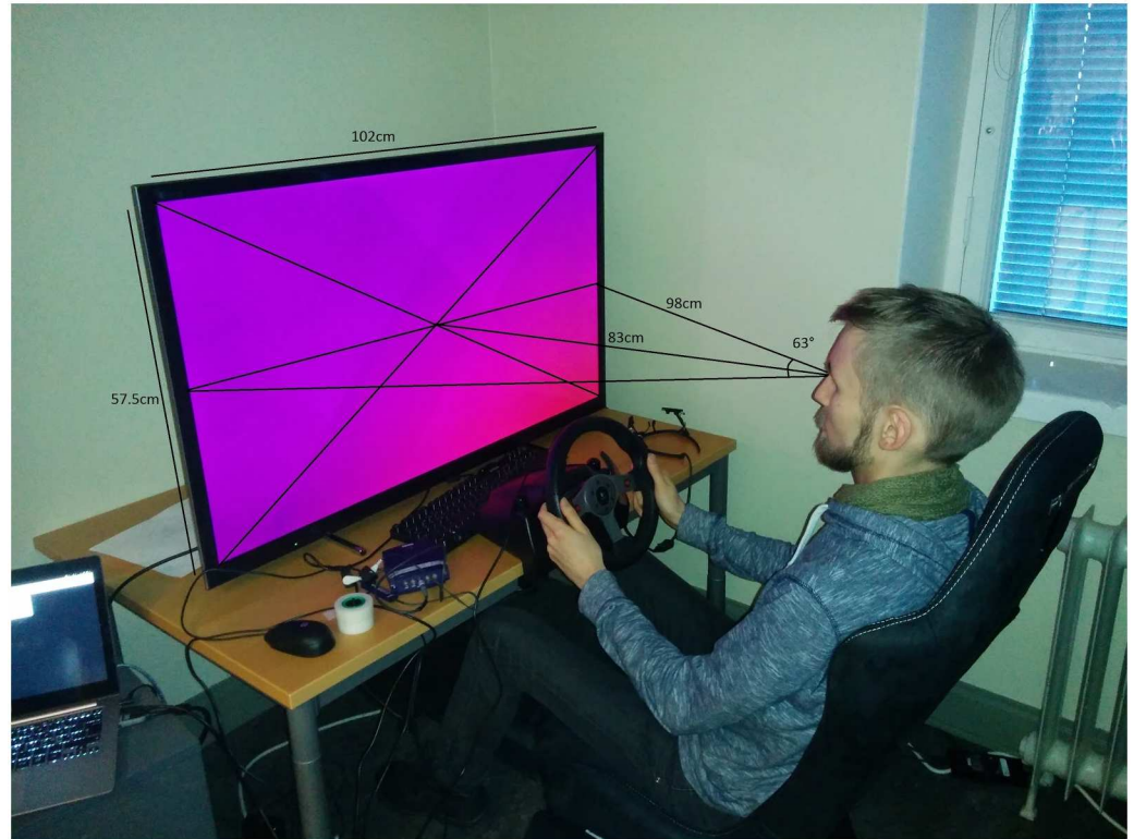
Fig 1. The physical setup of the driving simulator.
