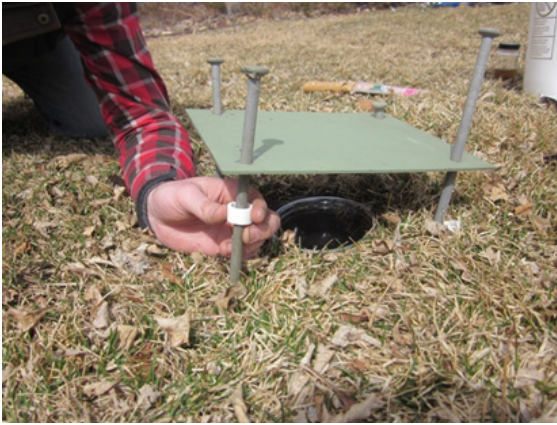
Fig. 3. A photo of a National Ecological Observatory Network pitfall trap mid-installation. The final design includes two nested cups, flush at ground level. In this photo, the technician highlights the short PVC spacers that elevate the hard plastic cover 1.5 cm above the trap entrance.
