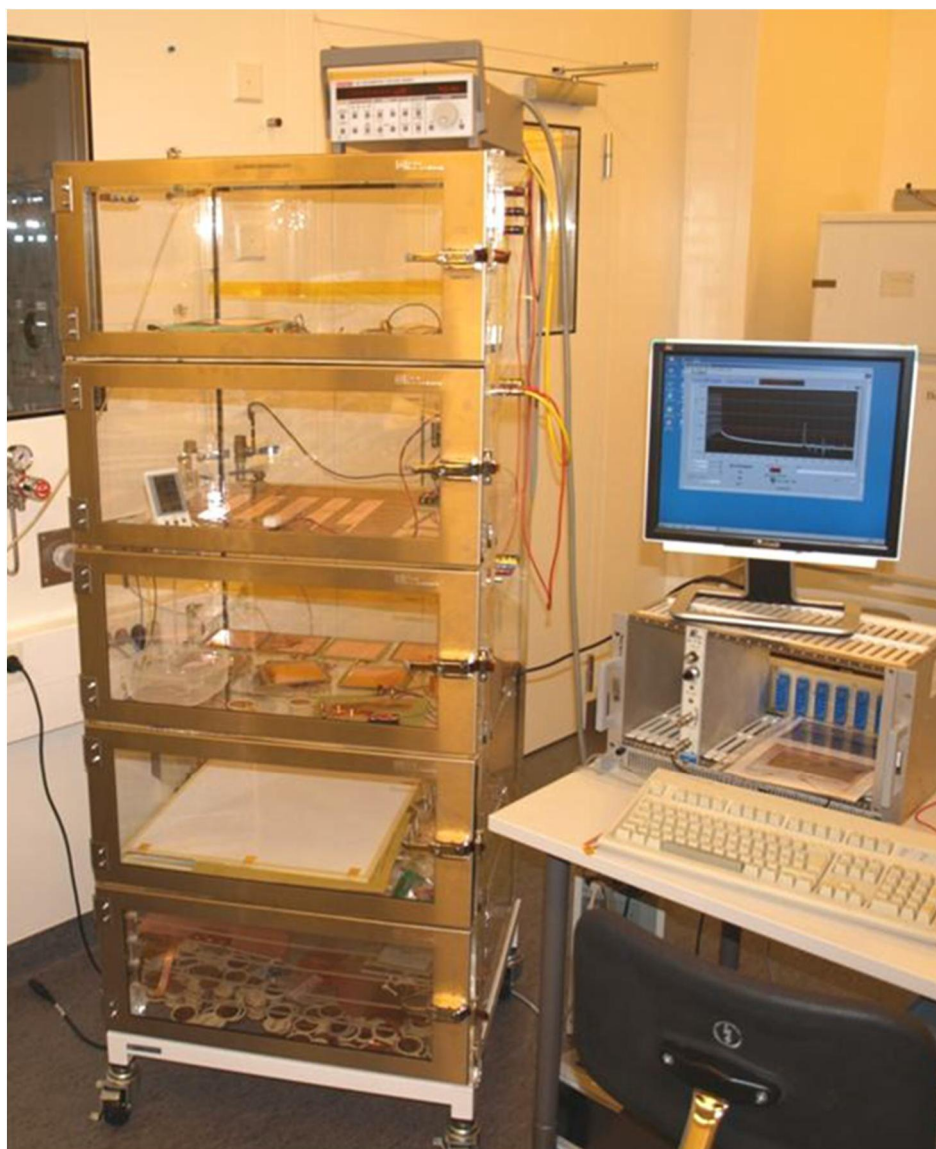
Figure 7.2: Leakage current measurement setup.
