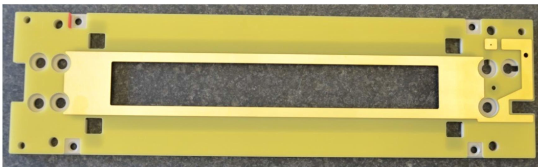
Figure 8.2: Picture of the field-terminating plate mounted on its backing.
