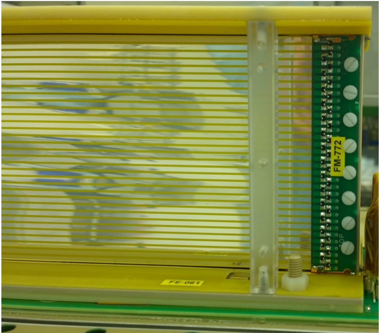
Figure 5.2: Field cage resistor divider.
