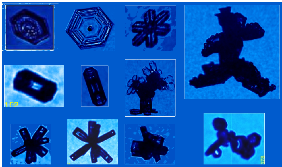
Figure 3: Examples of ice crystals measured by Cloud Particle Imager (CPI) installed on a measurement aircraft.
