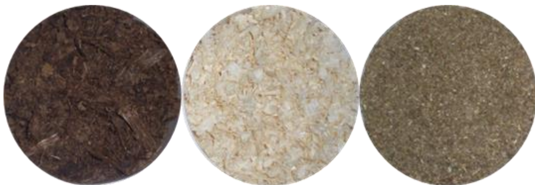
Photo 1 Bedding materials tested in broiler houses: peat, wood shavings and ground straw.
