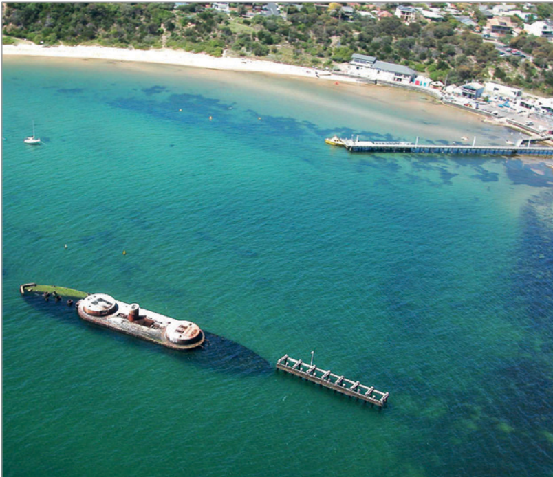
Fig 4.1. The pier and HMVS Cerberus as a breakwater (courtesy of Friends of the Cerberus ).
