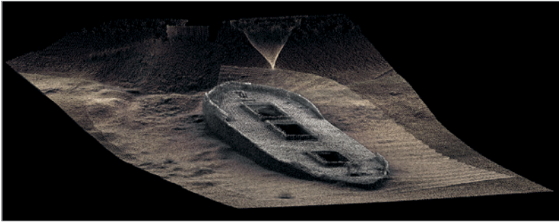
Fig. 4. The monitor, as scanned with the multibeam sonar equipment of Meritaito Ltd. (Picture: Ville Peltokorpi. Courtesy of the Governing Body of Suomenlinna).
