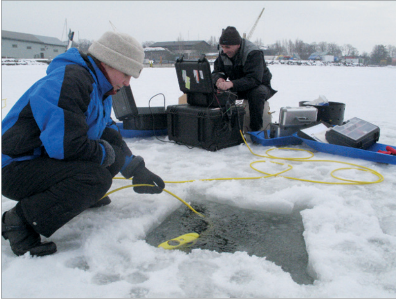
Fig 2.18. The wreck (ID 1312) is being checked with an ROV (Remotely Operated Vehicle) from the top of the ice. Pekka Paanasalo operates the equipment, and the author assists with the cable (Noora Hirvonen 2007, MA200706:10/National Board of Antiquities).
