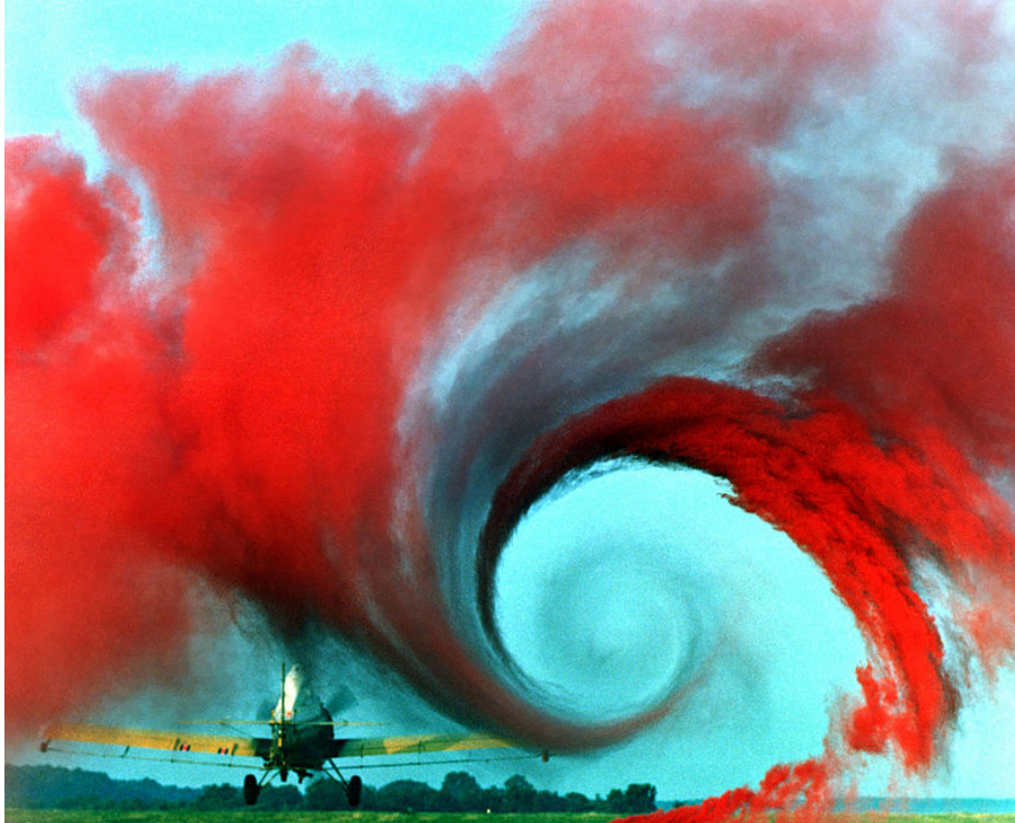
Figure 2.1. Wake Vortex Study at Wallops Island Flight Facility, VA, USA. Turbulent air flow created at the wingtips of an airplane in flight is made visible by red-colored smoke. Because such vortices (“dissipative” systems, as described below) are invisible to the naked eye, and can be fatal to airplanes that inadvertently fly into such turbulence, this phenomenon is studied in order to avoid such wake-vortex conditions at busy airports. NASA Langley Research Center (NASA-LaRC), Edited by Fir0002. Image in the Public Domain.
