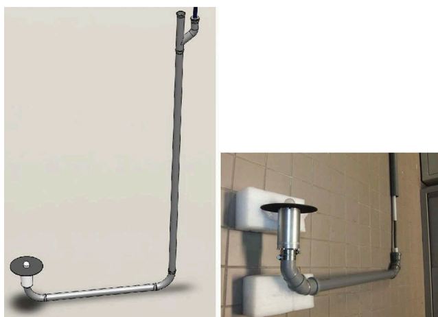
Fig. 2. Scheme of the apparatus developed for measurements of spectral underwater solar irradiance. Detail of the optical receiver and multilayer protecting frame of underwater device for measuring downwelling spectral irradiance.
