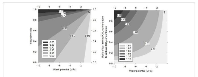
FIGURE 3 | Transpiration rate as a function of the saturation ratio S (S = RH/100%) and the water potential (A) and the CO<sub>2</sub> assimilation rate as a function of the CO<sub>2</sub> concentration in the internal (sub-stomatal/intercellular) cavity and the water potential (B), both gas exchange rates normalized to the flat surface value.
