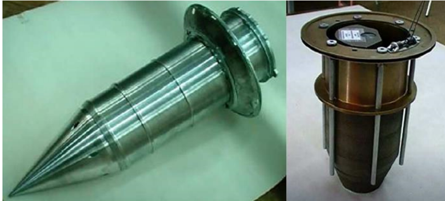
Figure 7. On the left is the surface module forebody deployed. On the right is the internal body together with equipment module mounted below it. Shock absorbing system tubes are visible. The hollow tubes absorb kinetic energy by deforming as they slide through too-small openings on the flanges of the internal body.
