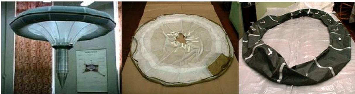
Figure 6. Inflated additional inflatable braking unit (T-IBU) shown on the left with the surface module (SM). In the centre the cover of the T-IBU and on the right the gas-tight bladder.
