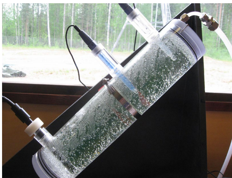
Fig. 5. On-line fluid monitoring during pumping. Attached to the flow through cell are (from left to right) a combined electrical conductivity (EC), O 2 and temperature sensor and sensors for measuring the redox potential and pH. The pumped fluid enters the cell from the bottom left end and comes out through the tube on the upper right end. Photo: Ilmo Kukkonen, University of Helsinki.
