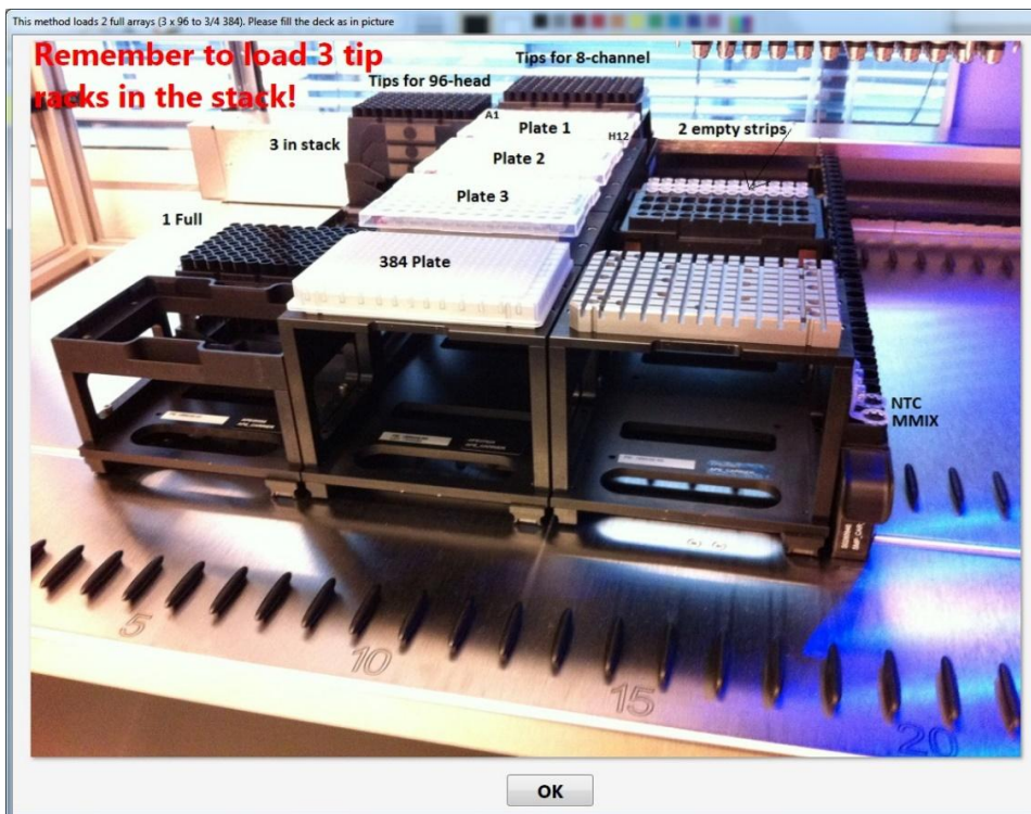
Figure 13. Hamilton Starlet: OpenArray96to384 program deck layout.
