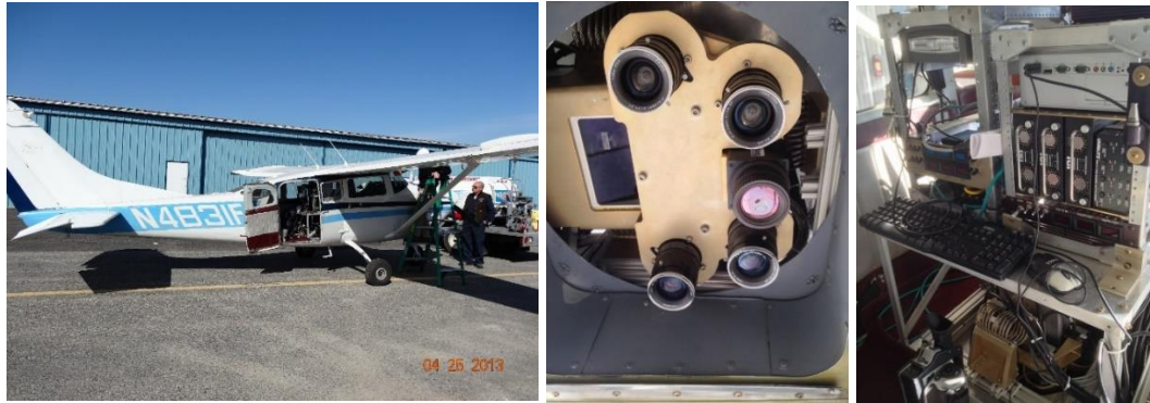
Fig. 4.2. The USU LASSI LiDAR and airborne multispectral remote sensing system including FLIR SC640 thermal IR camera installed in the Cessna TP206 remote sensing aircraft.
