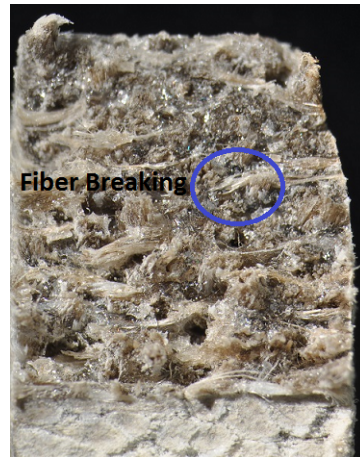
Fig. 6.9: Microscopic Image of Surface Morphology After Impact Failure of Flax/Epoxy Composite
