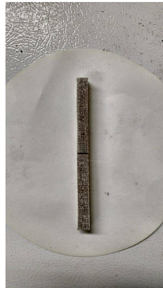
Fig. 6.6: Composite Sample After Sanding
