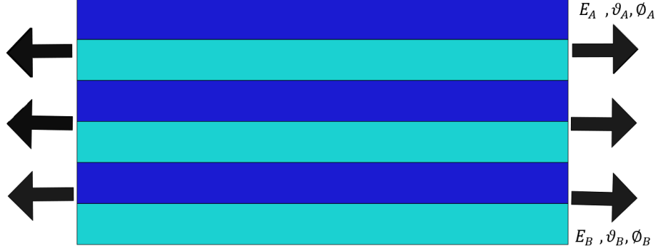
Fig. 5.2: A Schematic Diagram of a Layered Composite Under Longitudinal Tension (Parallel Connection)
