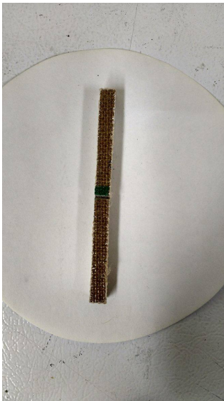
Fig. 6.5: Composite Sample Before Sanding
