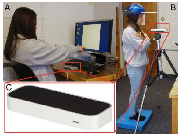
Figure 1 Test setup. for most tests (A), subjects pointed to objects on a screen while a Leap Motion sensor (C) captured their movements. In the balance test (B), subjects' head sway was extracted from the motion of dowels attached to a helmet.
