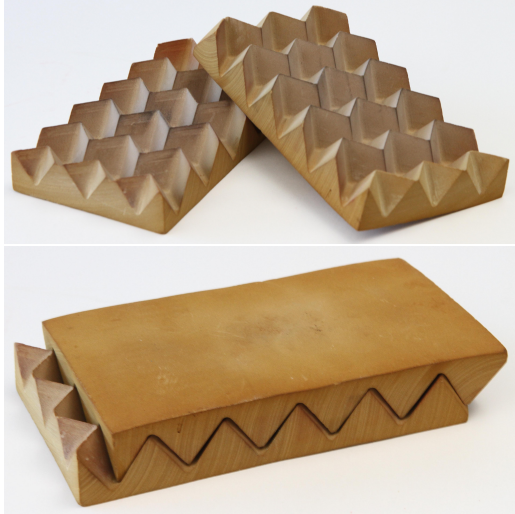
FIGURE 2: Two identical mold halves used for creating a Miura-ori pattern using the double mold process shown open and together
