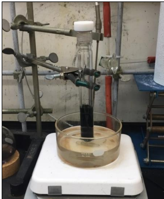
Figure 4: High pressure synthesis of ETT
