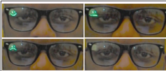
Figure 4. Actor wearing the display (image cropped); Clockwise: smile, neutral, turned off, frown.
