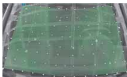
Fig. 3: Measured operational deflection shape (magnitude) at 116Hz with adaptive feedforward control (shaker excitation).
