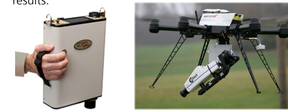
Figure 4: SVC 1024i field spectrometer (left) and Cubert Firefly snapshot spectrometer mounted beneath an ASCTEC UAV (right).
