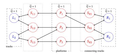
(b) Microscopic representation of the same station as in Figure 6.1a, with all platforms and physical tracks modelled explicitly.
