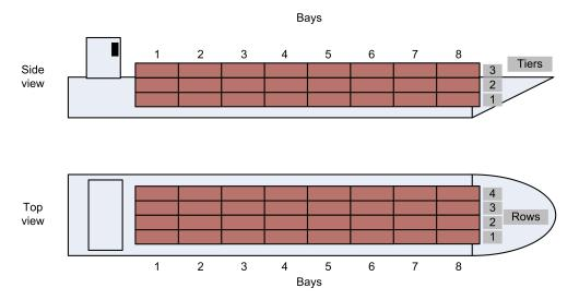
Figure 2.1: Conceptual container vessel
