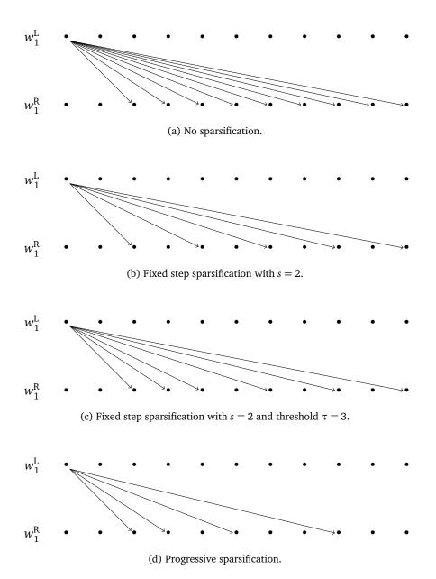
Figure 6.7: Graphical representation of various graph sparsification techniques on the time-space graph.
