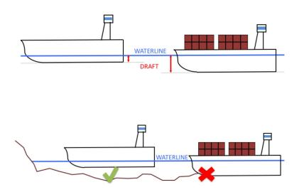
Figure 5.1: In the picture above, the draft of a ship as a function of the cargo on board. In the picture below, a ship able to enter a port (left) and one whose draft is too large to enter the same port (right).
