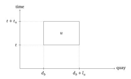
Figure 3.3: A representation of the planning horizon, showing a ship u docket at berth b from time t to time  $t + t_u$ .
