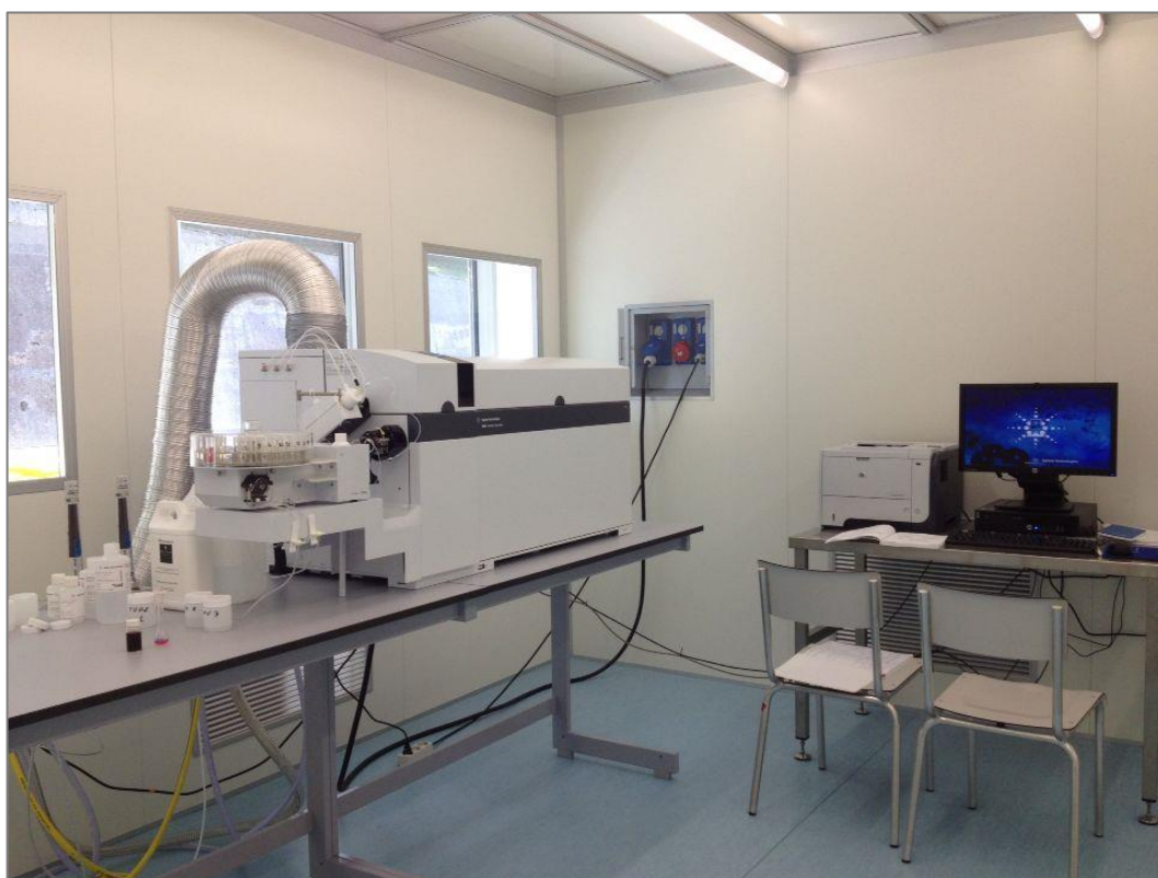
Figure 3.10 The inductively coupled plasma mass spectrometer (ICP-MS 8800 Agilent T.) installed in the Clean Room (ISO Class 6) in ENEA Brasimone Research Center.
