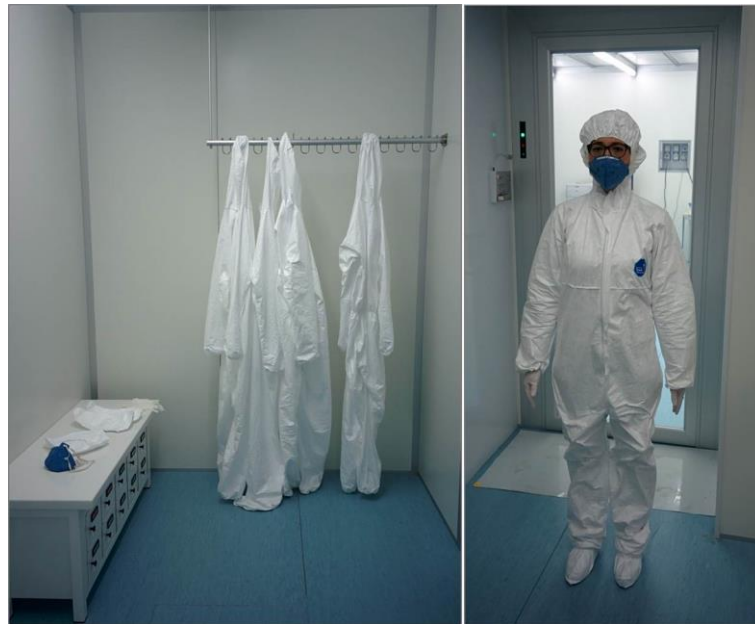
Figure 3.11 The operating personnel, dressed with all required accessories, before entering in the Clean Room (ISO Class 6) in ENEA Brasimone Research Center.
