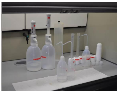
Figure 3.6 Clean Laboratory equipment: laboratory glassware in PTFE or PFA.
