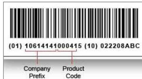
Figure 1.4 An example of alphanumerical codes divided in company prefix and product cod number.
