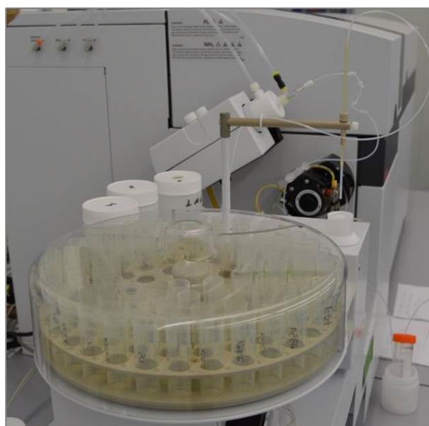
Figure 3.17 The Integrated Autosampler coupled with the ICP-MS installed in the Clean Room.
