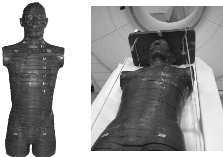
Figure 2.2 The Alderson RANDO phantom [4]. An anthropomorphic phantom, used in combination with TLDs to measure organ doses in Paper 2 of this PhD thesis.
