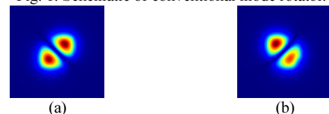
Fig. 2. The two orthogonal modes of the mode rotator.
