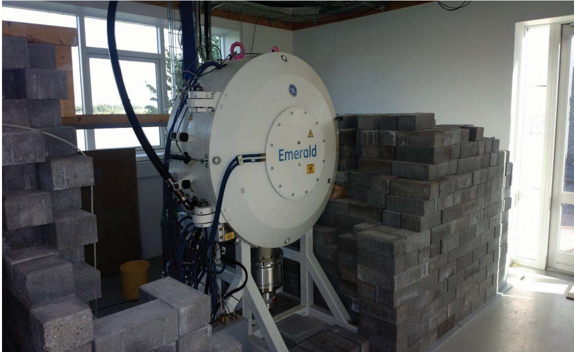
Figure 2 The prototype cyclotron photographed in operation – The right hand concrete bricks constitute the outermost layer of the target shield.
