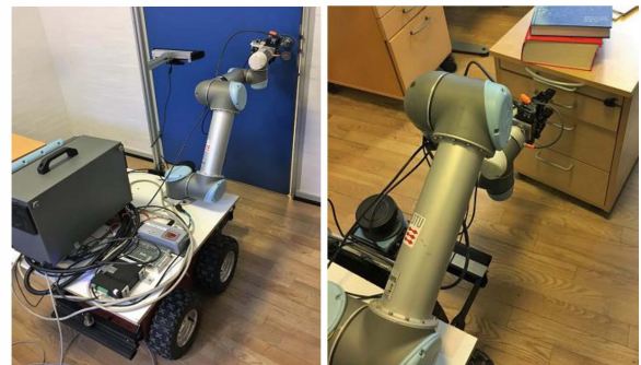
Figure 7. Mobile robot grasping door and cabinet (drawer) handles
