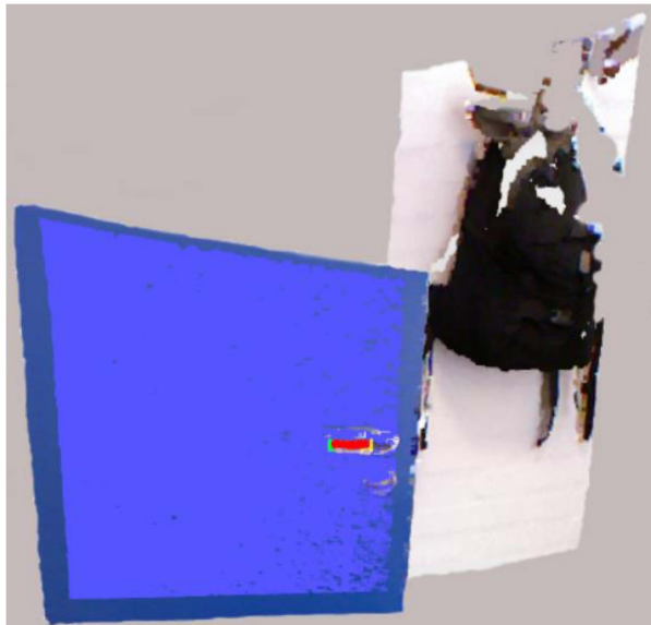
Figure 6. The handle (red) and door plane (clear blue) point clouds obtained after using both methods are layered on top of the full environments point cloud. This visual segmentation method for this case is seen in Figure 4 and the method fusion corresponds to Figure 5. The green and yellow points on the left and right side, respectively, of the handle point cloud are some of the key features required for future robotic manipulation.
