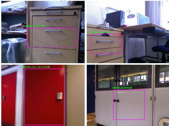
Figure 3. Resulting bounding boxes for several cabinets and doors. Their respective door and handle point clouds are depicted in Figure 8
