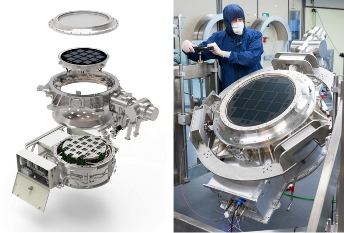
Figure 13. JPCAM 1.2 Gigapixel cryocam (a) exploded view (b) assembled instrument
