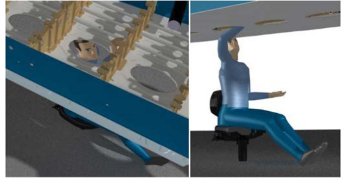
Figure 3. CATIA simulation of example posture adopted by operators during assembly task close to the man-hole.
