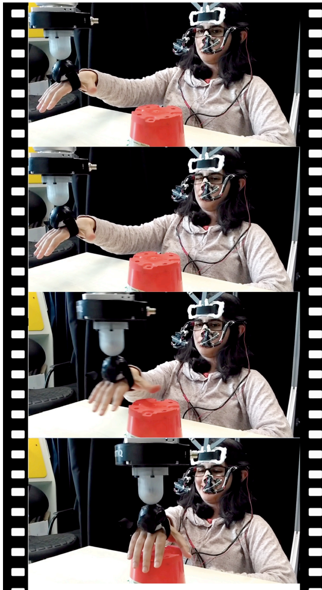
Fig. 1. Video snapshots of the system in operation. (1) The user looks at a target (red cylinder) while the 3D location of his gaze is continuously monitored by our GT3D eye tracker. (2) The user’s winks trigger the robot actuator to start moving (3) and, finally (4) stopping at the 3D location of the triggering moment’s gaze-target over the red cylinder enabling the user to grasp it.
