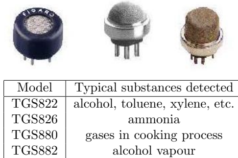
Figure 3: Top: Figaro gas sensors. Bottom: Sensors used and their selectivity characteristics.
