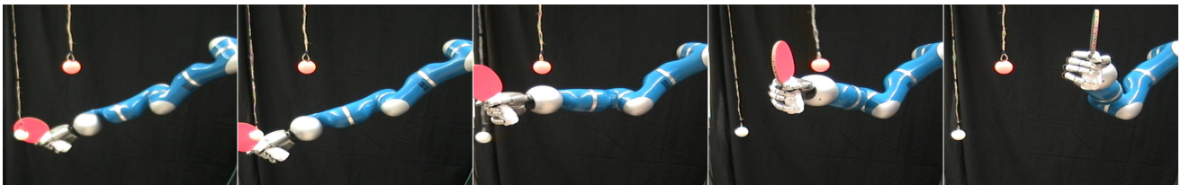
Fig. 8. The robot learned from demonstration how to hit one of two targets (indicated by the white and orange table tennis balls) while avoiding the other. The figure shows the combination of both movement primitives. By activating both primitives, the robot hit the white ball and subsequently the orange ball.
