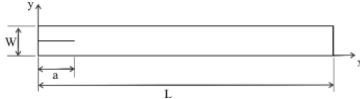
Fig . 5 Rectangular lamina with a crack
