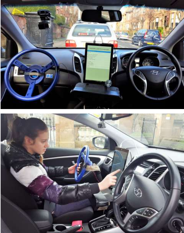
Figure 2. In-car experimental setup (top). A participant performing the scrolling task inside our vehicle (bottom).
