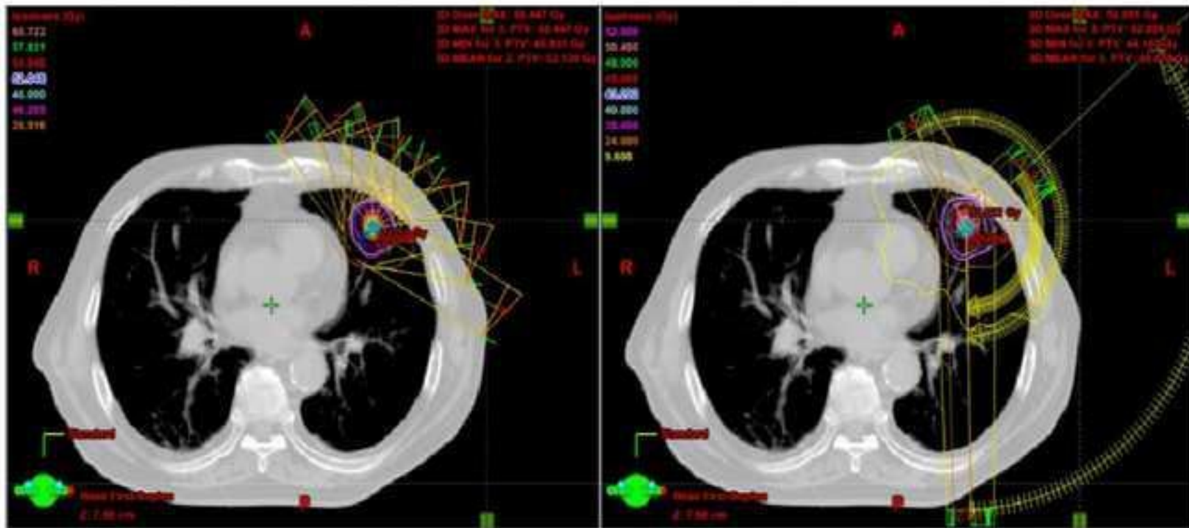
Figure 1. Typical 3DCRT and VMAT field arrangements used in the study. Left: 3DCRT field arrangement consisted of 9 beams, equally spaced, 20 degrees apart. Isodose distribution is optimized with the use of wedges. Right: VMAT field arrangement consisted of 3 non-coplanar partial arcs, with couch rotation of 0, 15 and 345 degrees respectively. Dose distribution is optimized using inverse planning.
