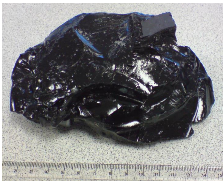
Figure 2.2: A piece of the MW25 weighing approximately 300 g. The scale on the ruler on the lower edge of the photograph is in cm (by courtesy of NNL, UK).
