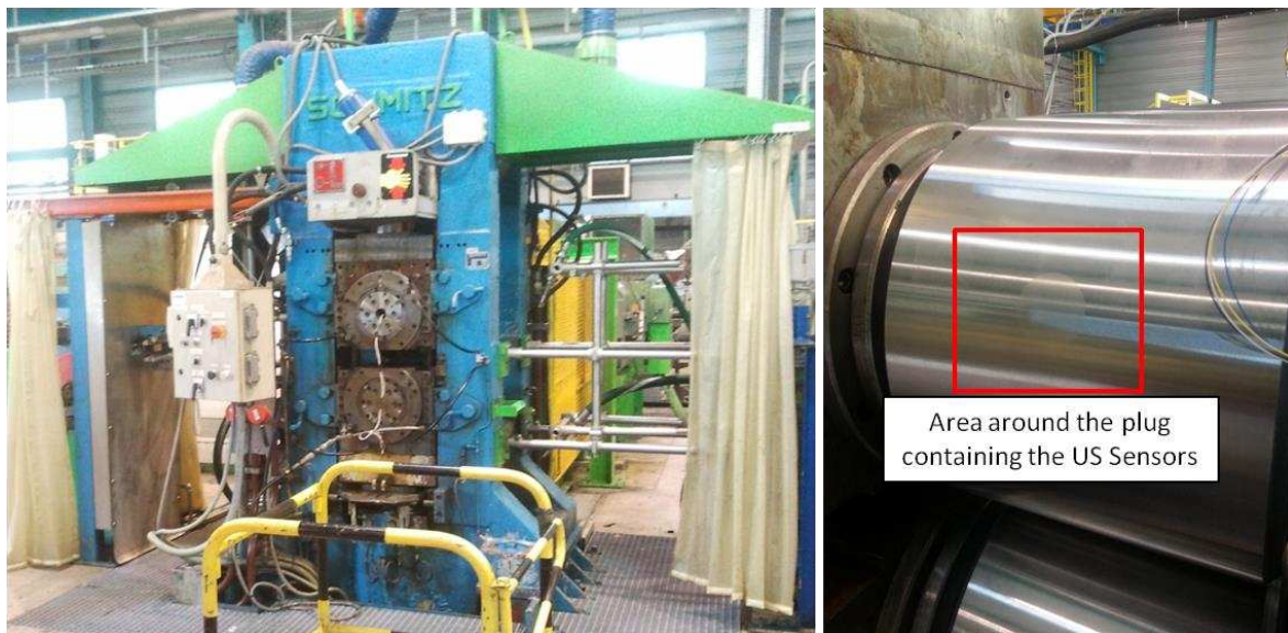
Figure 6. a) ArcelorMittal pilot mill where ultrasonic sensors were tested. b) Roll surface, around the plug containing the ultrasonic sensors, after grinding. The geometrical discontinuity is reduced and the plug position is barely visible.
