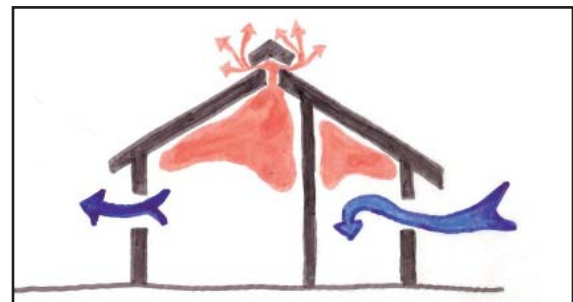
Figure 64: Cross ventilation without drop ceiling and partition wall. Notice elimination of cross ventilation and amount of trapped warm air.
