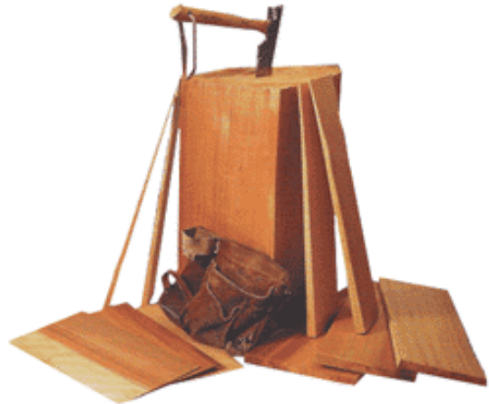
Figure 37: The traditional tools used to split wood shakes for roofing. Now machines are used to cut and split the wood shakes.
