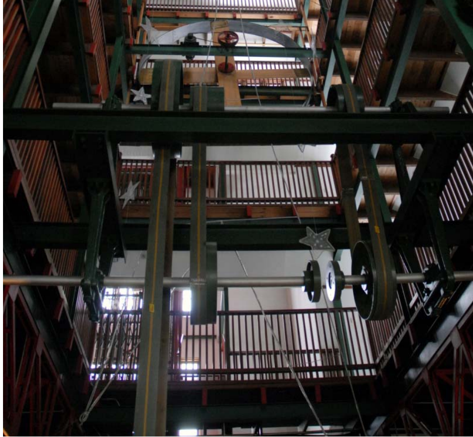
Figure 18. The Tea Factory Hotel contains a real, still working display of the mechanical drive-train system that, before, transferred tea leaves from one side of the factory to another. This makes an experience that is unique to the building, but not in a fashion of a Disney-fied ride or presentation. Today, the belts run at a slow speed. Source: http://www.flickr.com/photos/naeemebrahimjee/4817427991/sizes/o/in/photostream/
