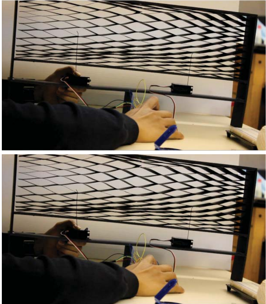
Fig. 5.61 - This image sequence is taken from a video showing the prototype being deformed to user interaction using the light-detecting sensor set-up.
