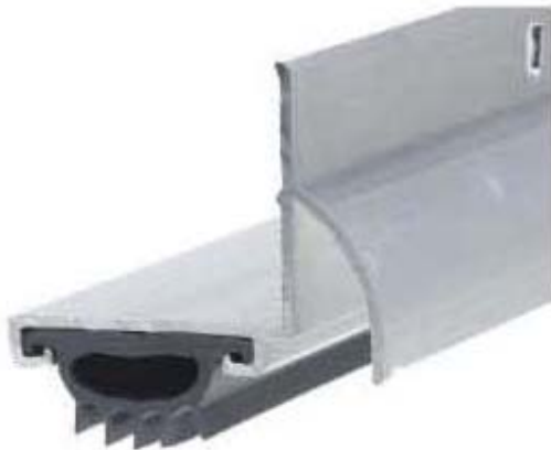
Example of an aluminum door sweep/door bottom with a rubber insert intended to be fastened on the outside with screws. This is intended for exterior doors as it also has a drip cap. Available at The Home Depot for about $8
