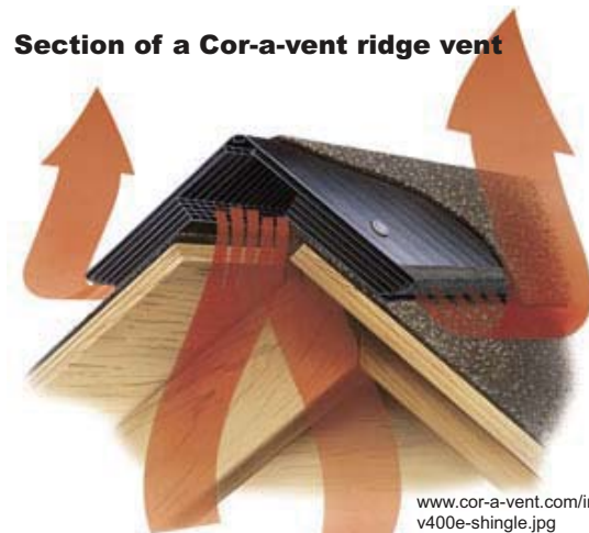
Section Diagram of a roof ridge vent showing how air can move up and out through the vent while at the same time keeping the roof water tight
