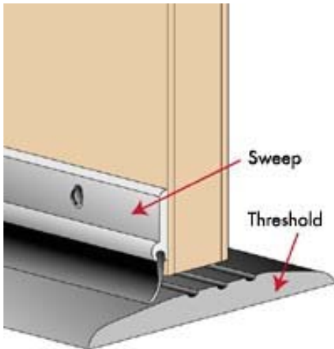
Diagram of a door sweep in relation to the door and threshold.
