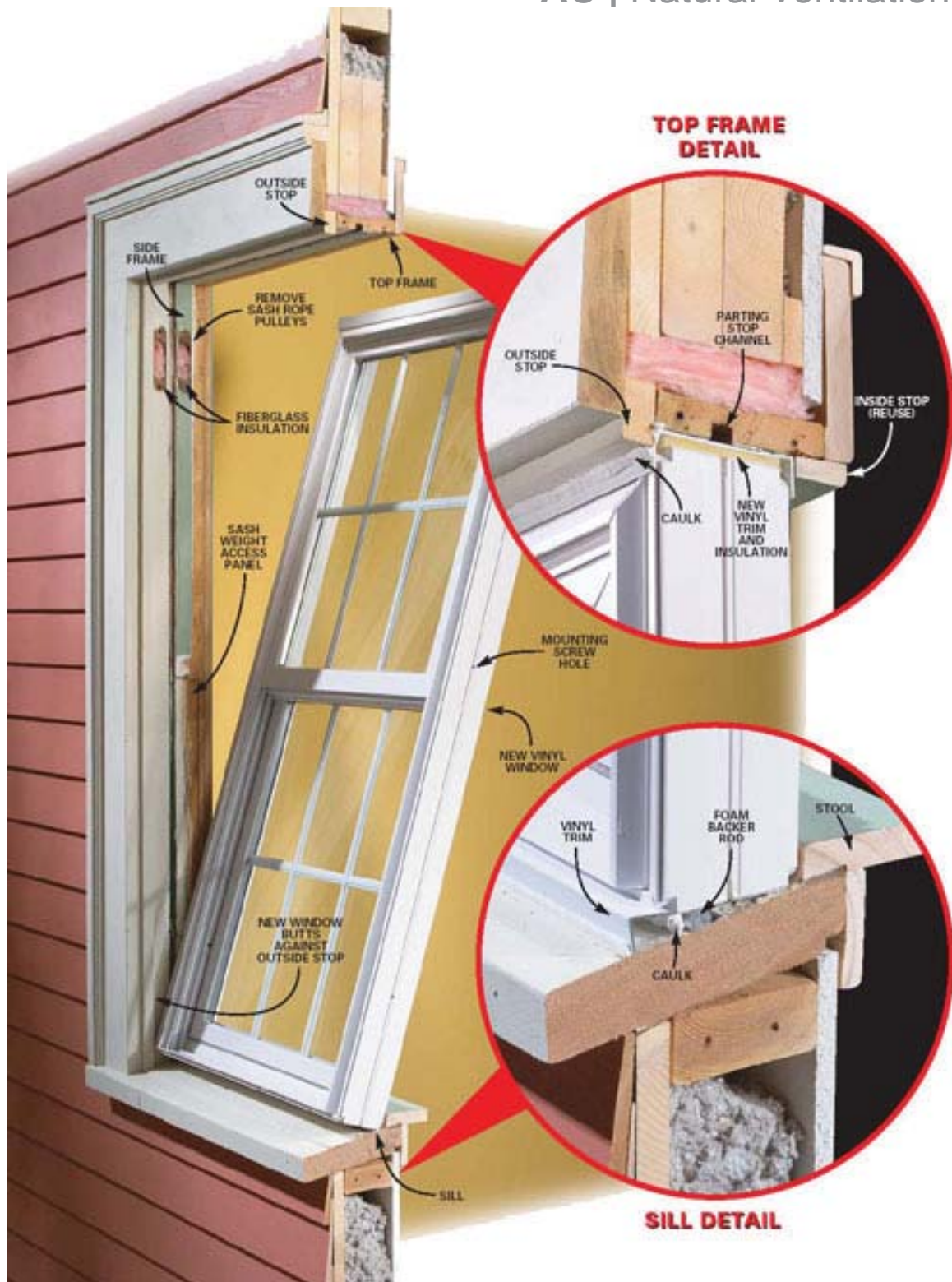
How to install vinyl windows, Diagram
