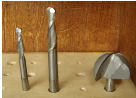
Figure 52 CNC router tool bits Left: 3/8" ball cutter; center: 5/8" ball cutter; right: 2" ball cutter
