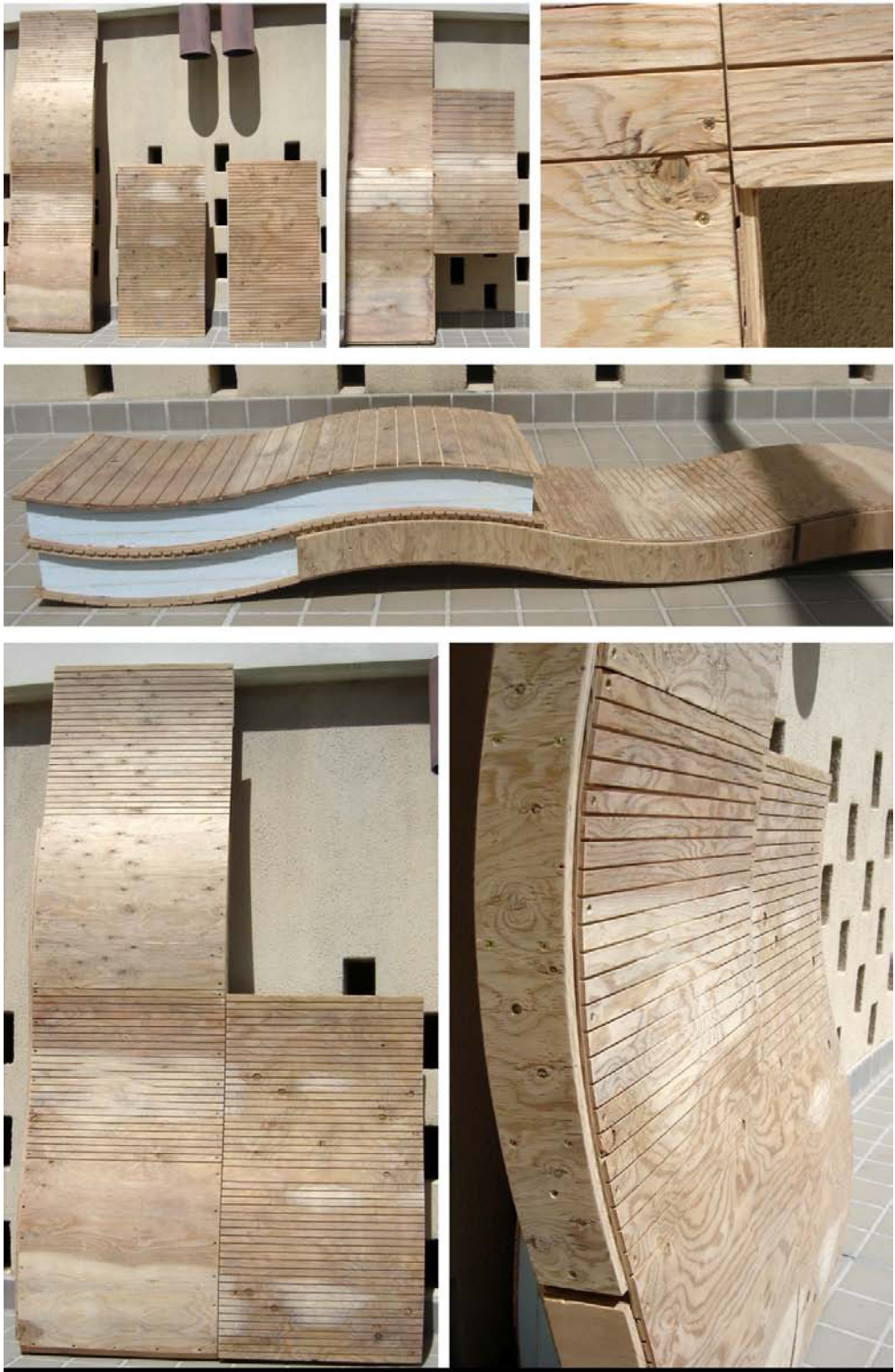
Figure 49 Vertical SIP wall assembly
