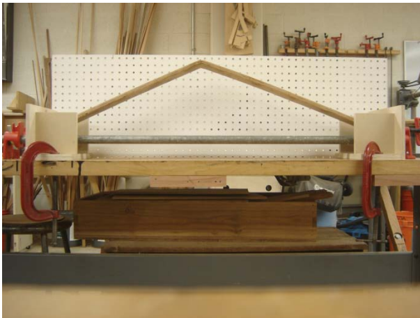
Figure 27 Five-ply. Five-layered plywood bending Test
