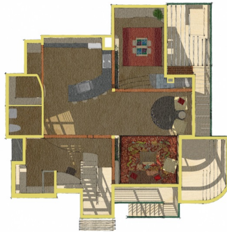
Figure 210. First Floor Transitional Space - natural light 3/21 at 11 am
