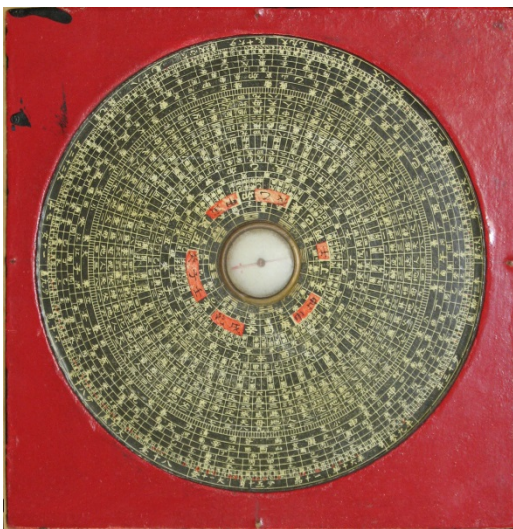
Figure 9. Chinese Compass – The Chinese compass is a magnetic compass that was used for orientation. The first ring around the magnetic compass has the eight trigrams from the yi jing . The surrounding rings have other information that
