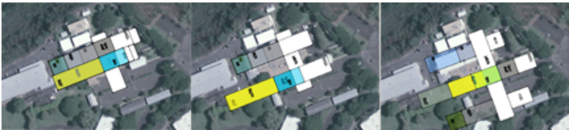
Figure 56. Three massing and configuration options: a. single building double width; b. 2 wings with connector space; c. 3 wings with connector space. Source: Google Earth
