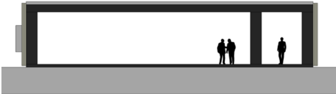
Figure 52. Building section showing open bay and enclosed office area created by structural elements. Source: SketchUp
