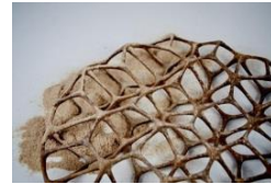
3D printed wood 20 (Integrated, generative design based on biomimetic approach)
