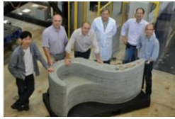
3D printed concrete bench 18
