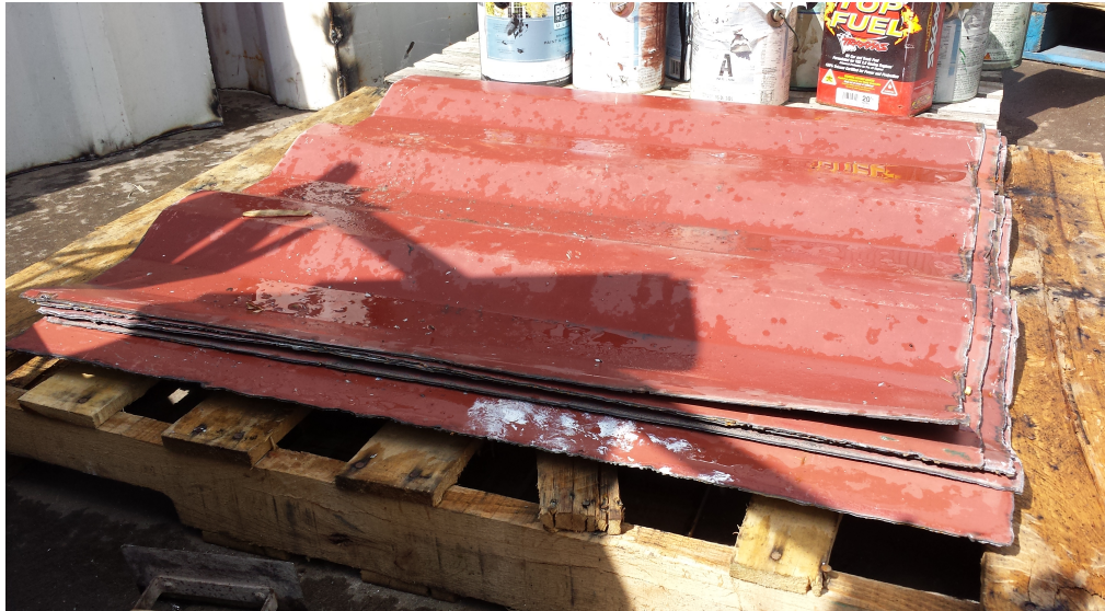
Figure 7.04-Pieces cut from shipping container to be welded together. Photograph by Richard E. Mead III
