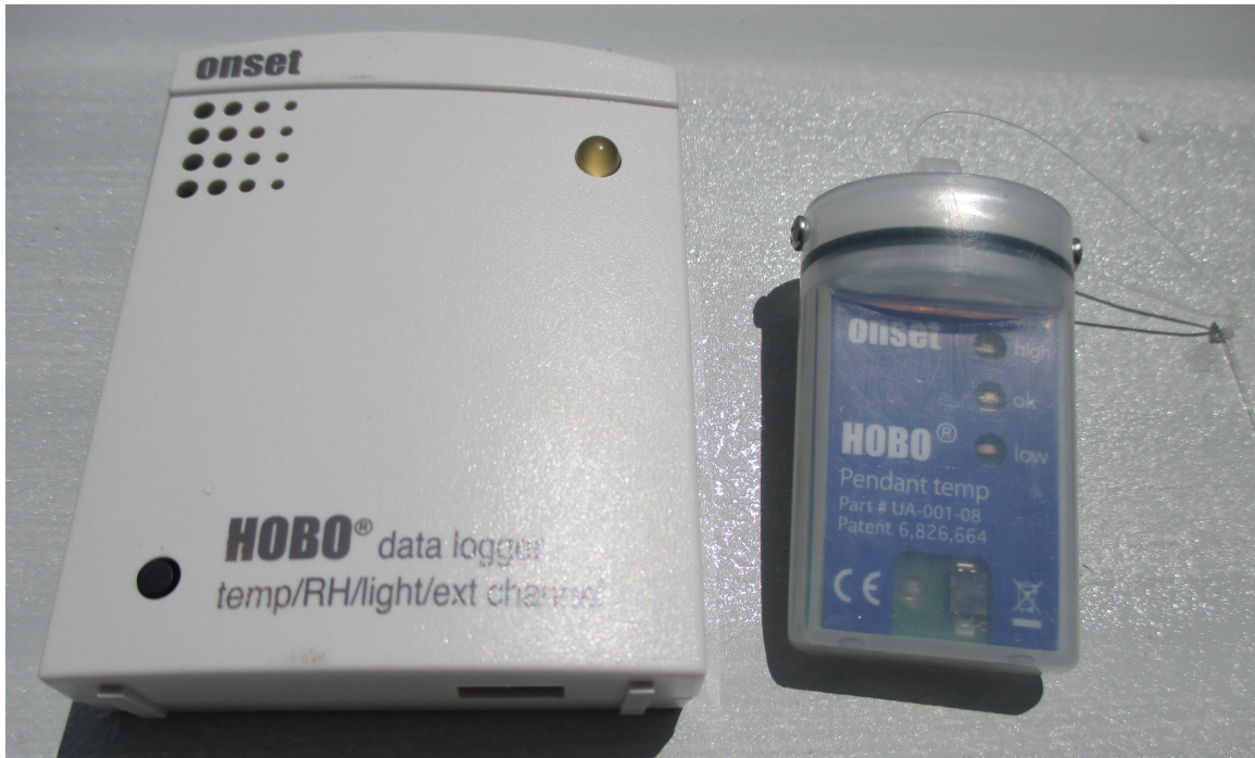
Figure 7.03- HOB0 data logger for interior temperature and relative humidity sensor. HOB0 onset exterior temperature sensor. Photograph by Richard E. Mead III
