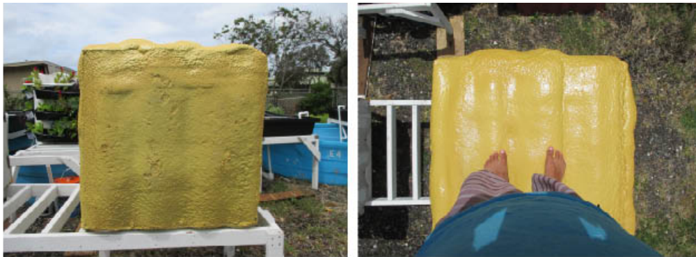
Figure 7.11- Closed cell spray foam box. Strong enough to hold up my weight while standing on top. Photograph by Richard E. Mead III
