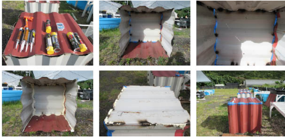
Figure 7.07- Materials used to seal the box and the process of taping the gaps to keep the foam in. Photographs by Richard E. Mead III
