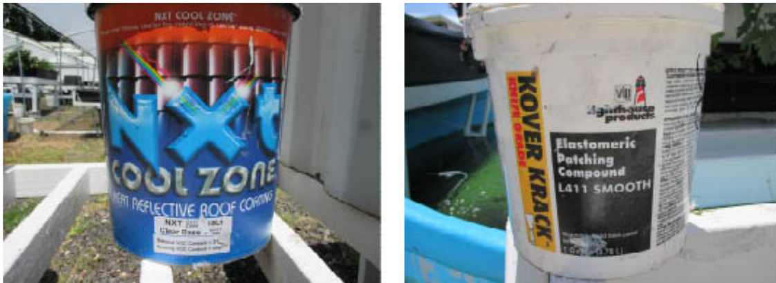
Figure 7.13 – NXT Cool Zone elastomeric paint and elastomeric patching compound. Photograph by Richard E. Mead III
