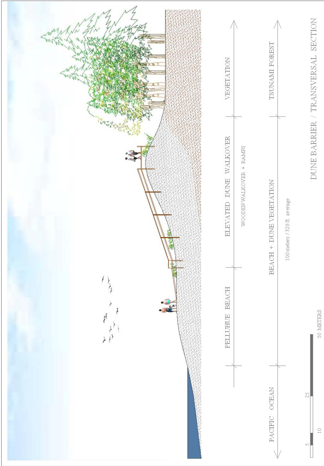
Figure 91: Dune Barrier / Transversal Section Source: Felipe Igualt 2014
